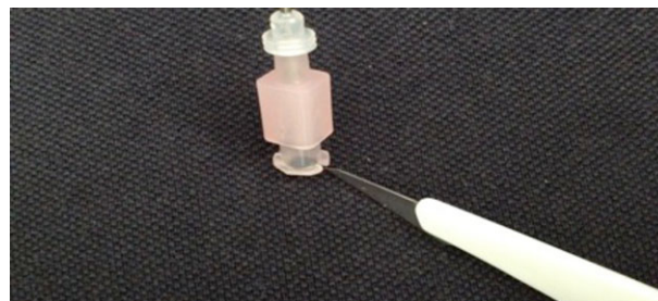
Fig. 1. Modified 18G needle showing newly created notch.
